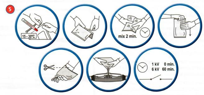
**1.13** For joints up to 1000v, joint can be filled under load conditions. The joint should be left for 2 hours before back-filling to allow resin curing process to begin.
