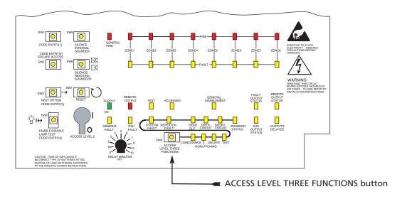
When the ACCESS LEVEL THREE FUNCTIONS button is pressed for the first time, the Accessed light will be lit steady and the first engineer function (COINCIDENCE) will be selected and indicated by its yellow light flashing (see right).
