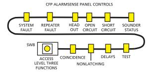
2. Continue pressing the ACCESS LEVEL THREE FUNCTIONS button until the SYSTEM FAULT light pulses.
