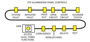
2. Continue pressing the ACCESS LEVEL THREE FUNCTIONS button until the REPEATER FAULT light pulses.
