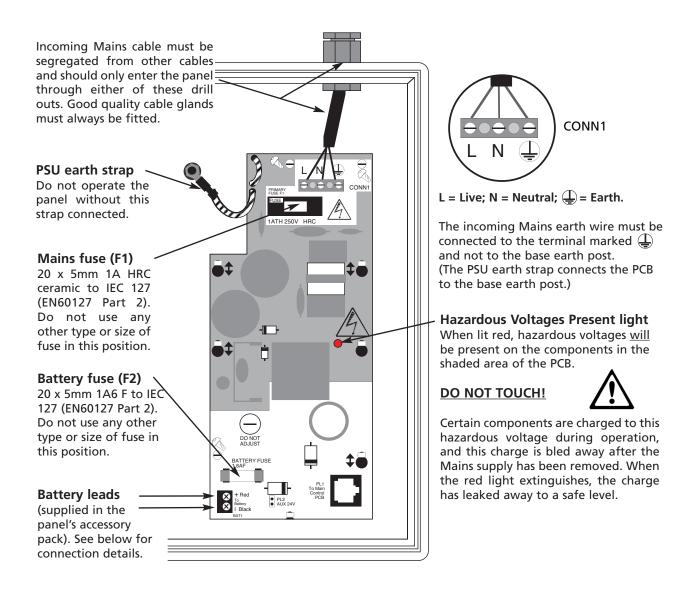
Figure 9 : Battery location and connection details
