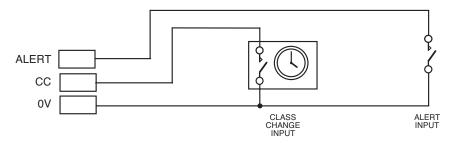
Connect the wiring for each input to the relevant 5mm connector block on the Main Control PCB and terminate their screens at the panel's base earth post (see page 13 for more details).
