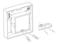
The MCP is installed by locating the upper mounting hook into the receiver in the back box and then pushing the unit gently home. The single fixing screw may then be tightened as required.
