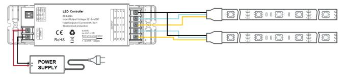
Application Circuit 3: RGB (V+ $\rightarrow$ COM, CH1 $\rightarrow$ R, CH2 $\rightarrow$ G, CH3 $\rightarrow$ B, CH4: NC.)
